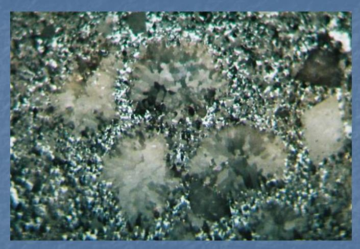
Example of bitumen infilling original porosity in oolitic limestone with ooliths subsequently replaced by calcite cement
