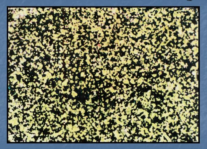
Example of bitumen infilling original porosity in carbonate – not very revealing!
